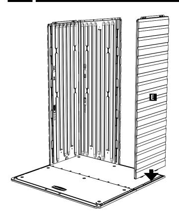
Using a screwdriver, punch out the screw holes on the top of Repeat Right Side (E) 2 places.
